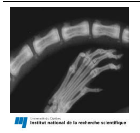
Fig. 2 Example of an absorption image obtained at Advanced Laser Light Source (ALLS at INRS -EMT, University of Québec). Distal hind limb and a tail of a mouse ~20 weeks old, 10 Hz laser at INRS, Mo target, Mo filter, SOD=30.0 cm, SDD=45.0 cm, intensity: 8 \times 10^{17} W/cm 2 , pulse duration: 70 fs, energy per pulse: 115 mJ, polarization: p , contrast: 10^{-10} , \lambda=400 nm, 4000 laser shots, hot electron temperature: 20 keV, Fuji EC-MA cassette/AD film used as an image detector.
